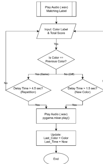
Figure 6. Audio playback logic flowchart
