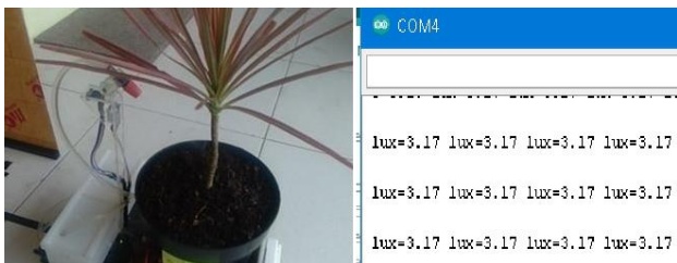
Figure 20. BH1750 Sensor Testing Results on Serial Monitor
